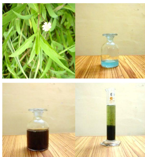
Figure 1: From left, kayyonni leaves ( Eclipta alba ), aqueous solution of Copper sulphate penta hydrate, the leaf extract and the formation of Cu-NP-KYN [5]
